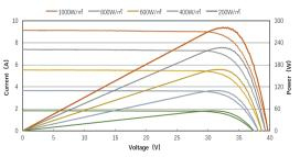
Excellent performance at 200W/m^2(AM 1.5, 25 C°): the conversion efficiency could be 96.6% of STC
