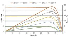
Excellent performance at 200W/m^2(AM 1.5, 25 C°): the conversion efficiency could be 96.6% of STC
